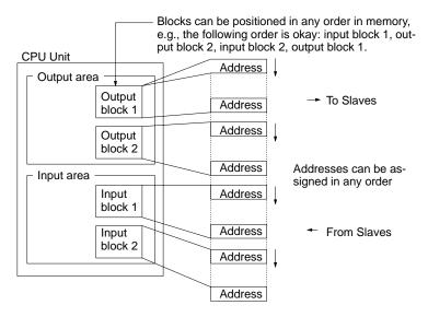
Words are freely allocated to the Slaves and I/O blocks can be set as desired. Each node must be allocated at least one byte (leftmost or rightmost). If a Slave requires more than one input or one output word, then it can be allocated more than one input or output word. If a Slave requires less than one word, it will use either the rightmost or leftmost bits in the word allocated to it.
